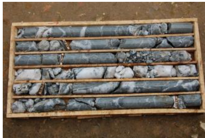
Photograph 2: BDDH002 from 55m to 60m showing silica veining, weak brecciation and disseminated pyrite.
