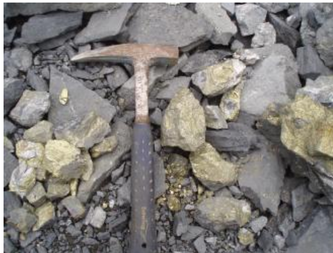
Photograph 5: showing chalcopyrite on the ore dumps outside the Shuilong Mine Adit.
